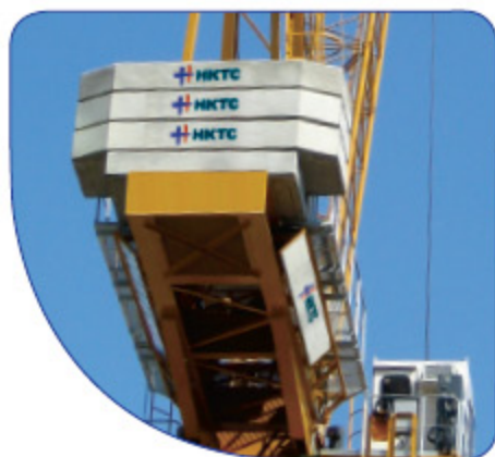
COUNT JIB & BALLAST BLOCK
