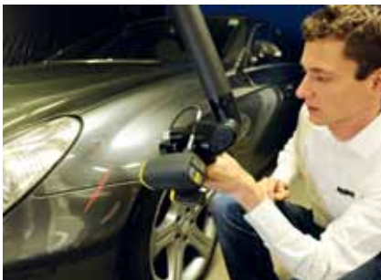
MMDx scanner is available in 50/100/200mm stripe width and MMCx features a 80/160mm stripe width
