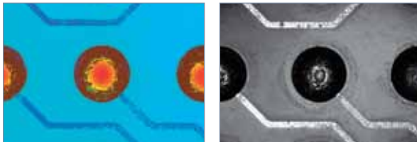
Confocal images captured by Z scan are reconstructed in real time into 3D contour map and EDF (Extended Depth of Focus) images.
