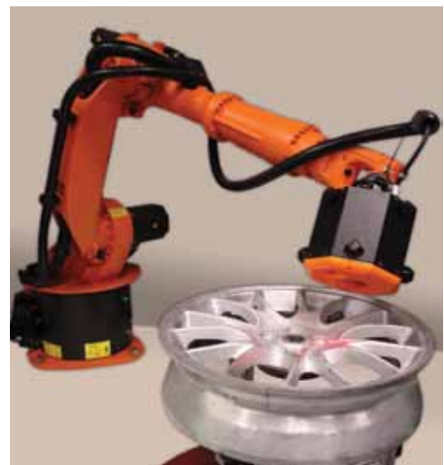
Fast repetitive laser scanning for in-production-line inspection
