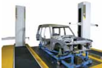
LK H-R dual column horizontal arm CMM
