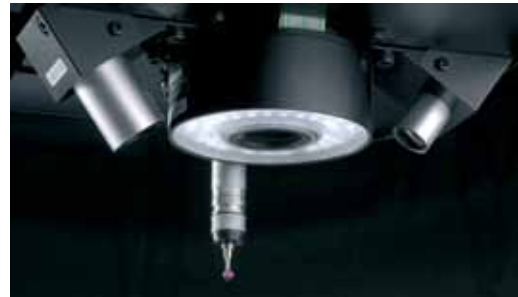
Multi-sensor capability makes surface and side coordinate measurement of complicated 3D parts possible
